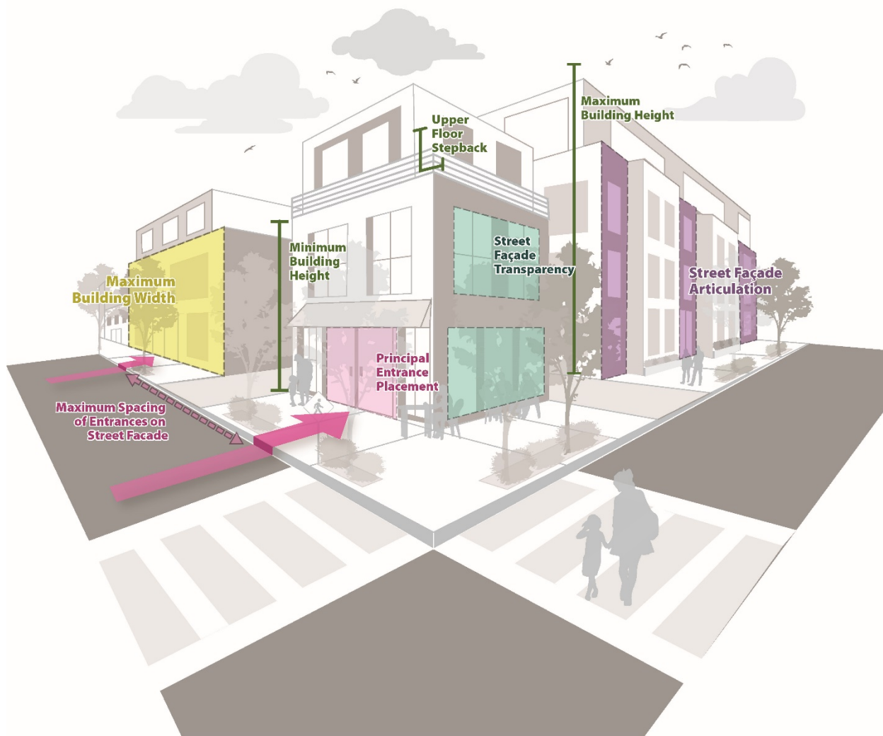
Figure 10. Building Design Element Illustration
